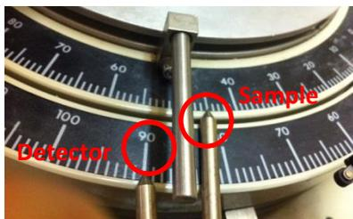
2. Check the Chi and the Phi. They should be at 0 (zero).
