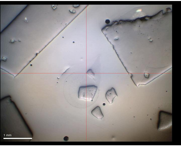
This is the zero point photographed at the same magnification (e.g., 20x objective with 10x ocular) u s ed to log target coordinates and similar to the field of view on the SIMS microscope targeting system (see pg. 14). The digital stage is set to 0,0 h ere, and target coordinates are logged relative to this point.
