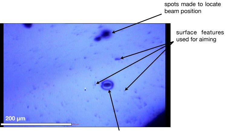
15 micrometer spot after analysis. Cesium deposition and "beam damage" to the coating around the pit causes the spot to appear larger than 15 micrometers.
