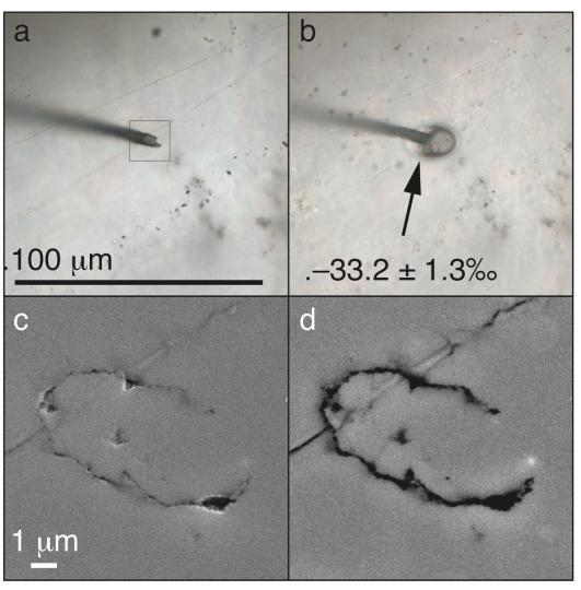
Screen capture from the SIMS microscope targeting system (field of view  $\approx$  450 µm) showing 15 micrometer spot after analysis. Note the difference in image quality between the SIMS optical system and a dedicated reflected light microscope (pg. 1-2), a factor that can contribute to difficulty in targeting during the analytical session.
