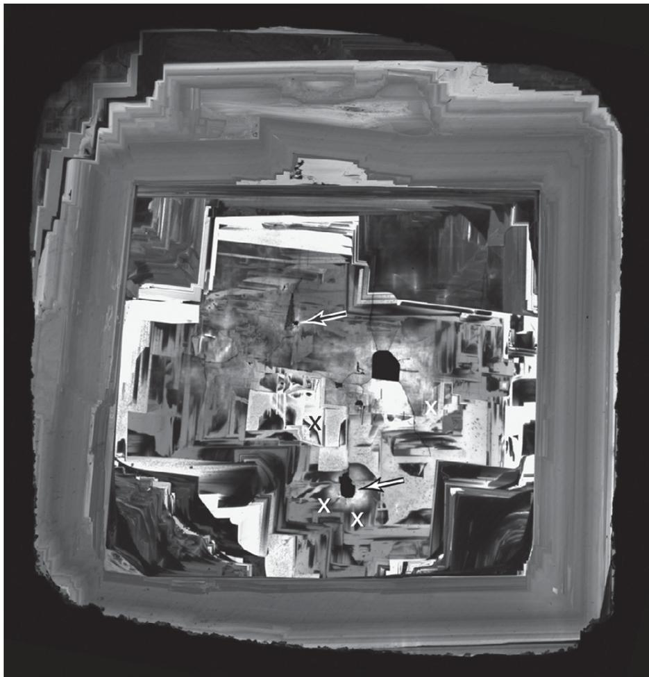
**Figure 1.** Cathodoluminescence image of diamond 13-127-16 from Guaniamo, Venezuela. Intensity of luminescence differs primarily due to nitrogen content of different growth zones. Silicate inclusions (two coesites, two omphacites, and one kyanite) appear as nonluminescent (black) regions. Locations of the two coesites analyzed in this study are indicated by arrows, and locations of the spots analyzed for carbon isotopes are indicated by x. Diamond is ~2 mm across.
