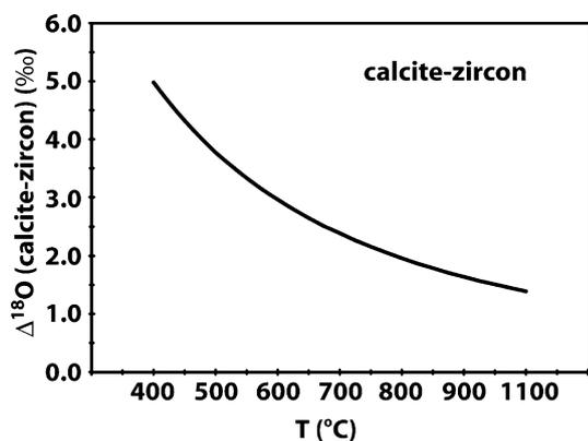
**Fig. 6** Oxygen isotope equilibrium for calcite-zircon. The calcite-zircon fractionation factor is from Valley (2003)
