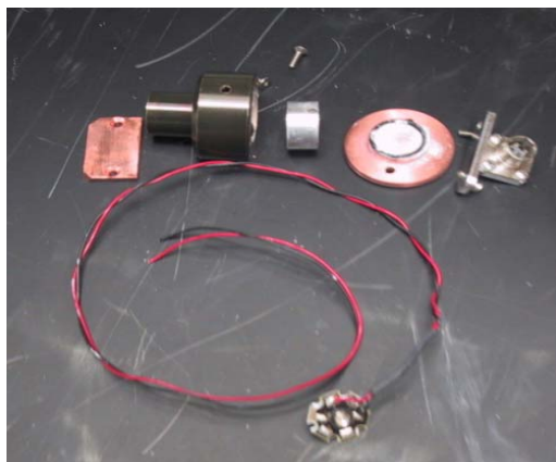
Disassembled Blue LED Illuminator assembly.
