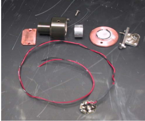
Disassembled Blue LED Illuminator assembly.
