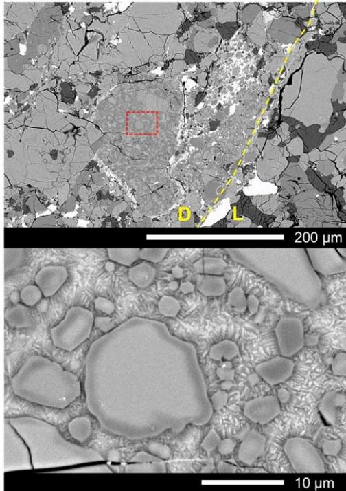
Fig. 3. Top: Boundary between a light clast (L) and a dark matrix (D), shown as a dashed line. The dark matrix contains melt clasts. The red square indicates the area shown in the bottom view. Bottom: Expanded image of a melt clast containing zoned olivine grains. Dark zones correspond to Mg-rich olivine ( $\sim\text{Fo}_{82}$ ). The mesostasis of the melt clast contains sub- $\mu\text{m}$  dendritic microcrystallites possibly with pyroxene composition.
