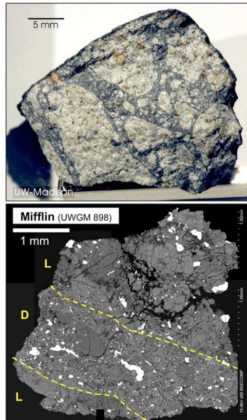
Fig. 2. Top: Mifflin meteorite, showing light clasts/dark matrix brecciated textures. Bottom: BSE image of a fragment of the meteorite, which shows a dark matrix (D) between two light clasts (L). Two dashed lines indicate the boundaries between two lithologies.
