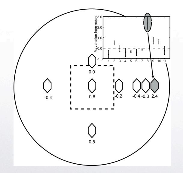
No fractionation across mount until extraction aperture overlaps the mount edge
