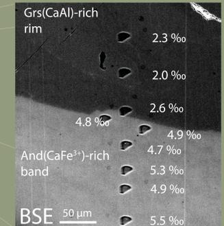
Figure 4. Back-scattered electron (BSE) image of ion-probe pits across the boundary between a high-δ<sup>18</sup>O, Fe<sup>3+</sup>-rich band and a low δ<sup>18</sup>O, Al-rich band. δ<sup>18</sup>O values are corrected as in Figure 6, and are approximate.
