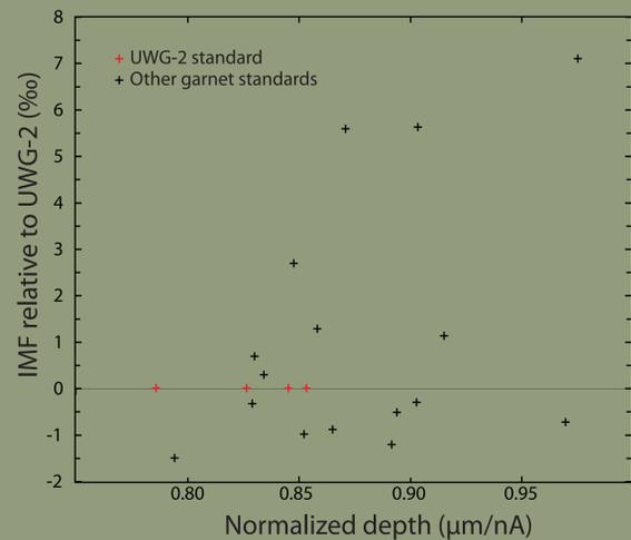
Figure 1. It has been proposed that IMF may be caused by differential sputtering rates (Eiler et al., 1997). In order to evaluate this, a sputter test was conducted using the WiscSIMS IMS-1280 in a 10x10μm raster mode. Pit depths were measured with a Zygo white-light profilometer and normalized to the average primary current during sputtering. No correlation is observed between pit-depth and IMF.
