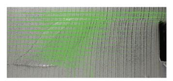
Particle Integrated Velicometry is an easy to implement system that permits tracking of indvidual particles through the experiment. Here is a PIV for one step in the restraining bend experiment.
