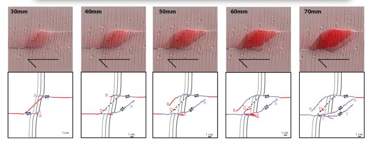
Fault evolution around a restraining bend in wet kaolin with 60% w.c. by weight. The laser scanned surfaces reveal the evolving topography of the clay surface.
