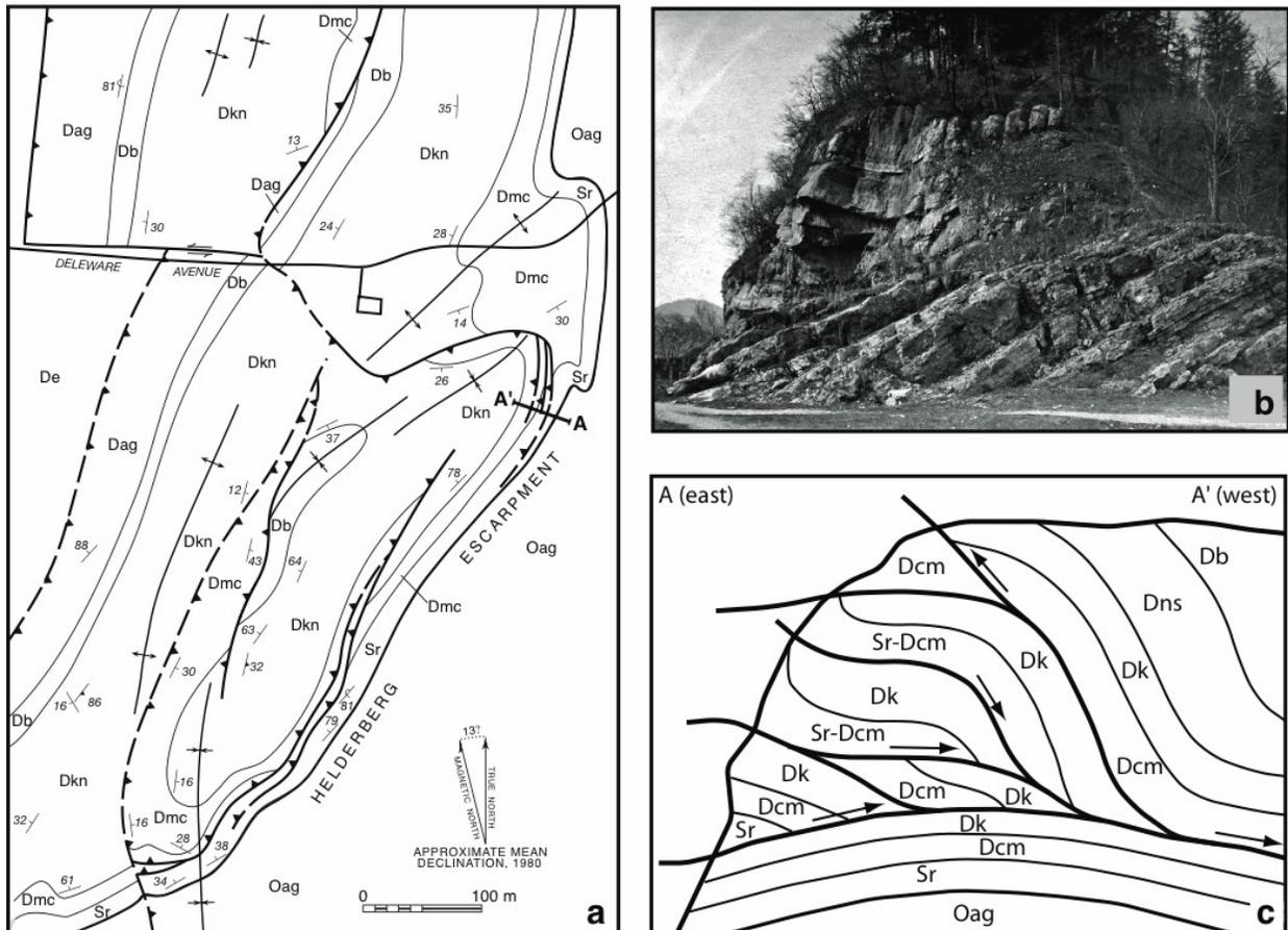
**Figure 11.** (a) Simplified geologic map of Hasbrouck Park (after Marshak and Tabor, 1989). Note complex structural relationships along eastern map margin. (b) Photo by G. van Ingen in Cairnes (1920) shows the NE corner of the escarpment in the park before regrowth of the forest. (c) A schematic cross-section above (not to scale), showing an imbricate thrust interpretation along Line AA'.
