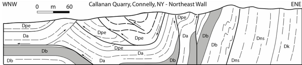
**Figure 12.** Sketch of the northeast highwall in the Callanan quarry in Connelly, south of Esopus Creek. Note the backthrusts and the steep dips. (From Marshak and Tabor, 1986, modified from an unpublished version by P. Kwizinski, UIUC M.S. student.)
