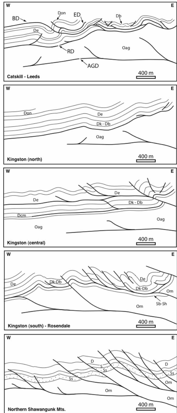
**Figure 6.** Model cross sections of the Hudson Valley fold-thrust belt at different latitudes (north at the top, to south at the bottom). Oag = Austin Glen; Om = Martinsburg; Sr = Rondout; Sb-Sh = Binnewater and High Falls; Dm-Dc = Manlius and Coeymans; Dk- Db = Kalkberg, New Scotland, and Becraft; De = Esopus; Don = Onondoga (Marshak and Tabor, 1986; Burmeister, 2006).
