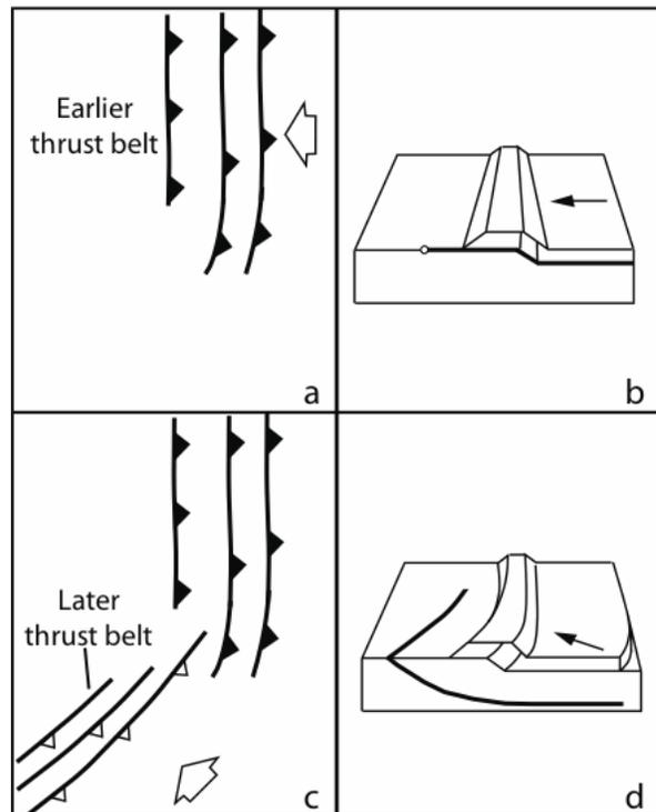
**Figure 4.** Block diagrams showing the concept of an intersection orocline. The NE-SW-trending thrust belt is younger than the N-S-trending thrust belt. Displacement on a younger thrust bends the structures in its hanging wall (Marshak and Tabor, 1986).
