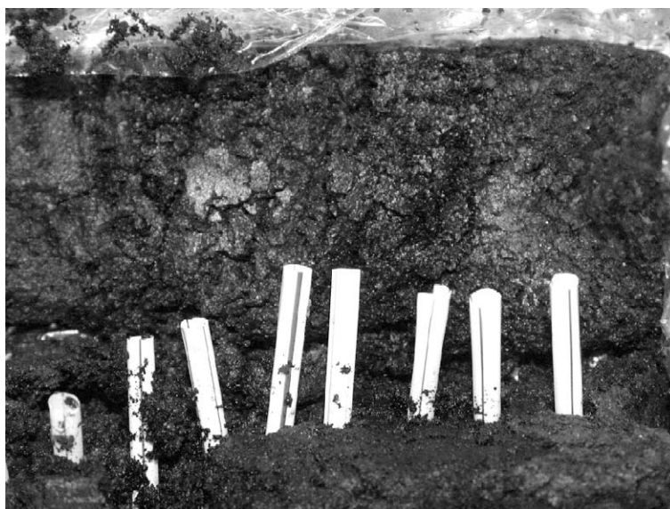
Fig. 6. Photograph of the upper 10 cm of the guano core. The drinking straws mark the position of the individual samples.
