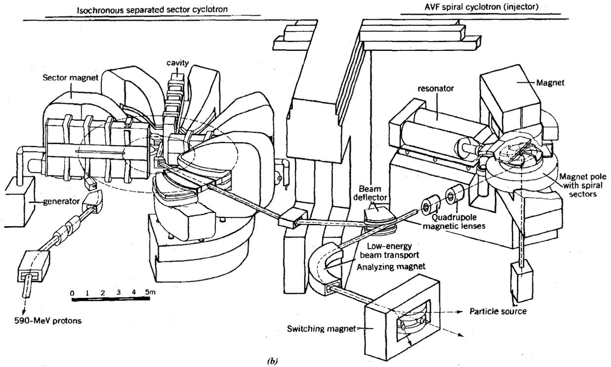
**Figure 15.13** SIN Cyclotron. (a) Scale drawing, showing injector AVF cyclotron with spiral extensions of magnet pole and separated sector cyclotron with spiral field boundaries. (b) Overhead view of field boundaries in separated sector cyclotron with calculated proton orbits at 75, 177, 279, 381, 483, and 585 MeV. (Courtesy W. Joho, Swiss Institute for Nuclear Studies.)
