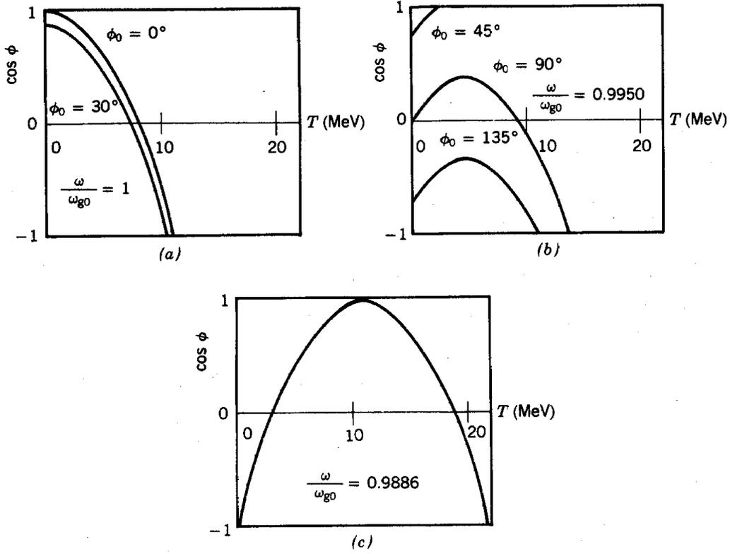
**Figure 15.5** Phase histories of protons in uniform-field cyclotron;  $\cos \phi$  versus kinetic energy ( $T$ ) for different injection phase ( $\phi_0$ ). (a)  $\omega/\omega_{g0} = 1$ , where  $\omega$  is rf angular frequency and  $\omega_{g0}$  is nonrelativistic gyrofrequency. (b)  $\omega/\omega_{g0} = 0.9950$ . (c)  $\omega/\omega_{g0} = 0.9886$ ,  $\phi_0 = 180^\circ$  (parameters for maximum kinetic energy).
