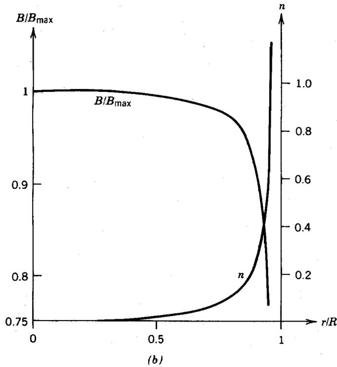
**Figure 15.2** Magnetic fields of uniform-field cyclotron. (a) Sectional view of cyclotron magnetic poles showing shims for optimizing field distribution. (b) Radial variation of vertical field magnitude and field index. (M. S. Livingston and J. P. Blewett, *Particle Accelerators*, used by permission, McGraw-Hill Book Co.)
