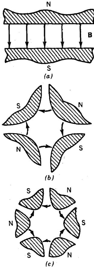
**Figure 15.15** Classification of synchrotron magnets. (a) Dipole magnet (bending particle orbits). (b) Quadrupole (transverse focusing). (c) Sextupole (chromatic correction; assuring that particles in a range of energy about the mean have the same  $\nu$ ).
