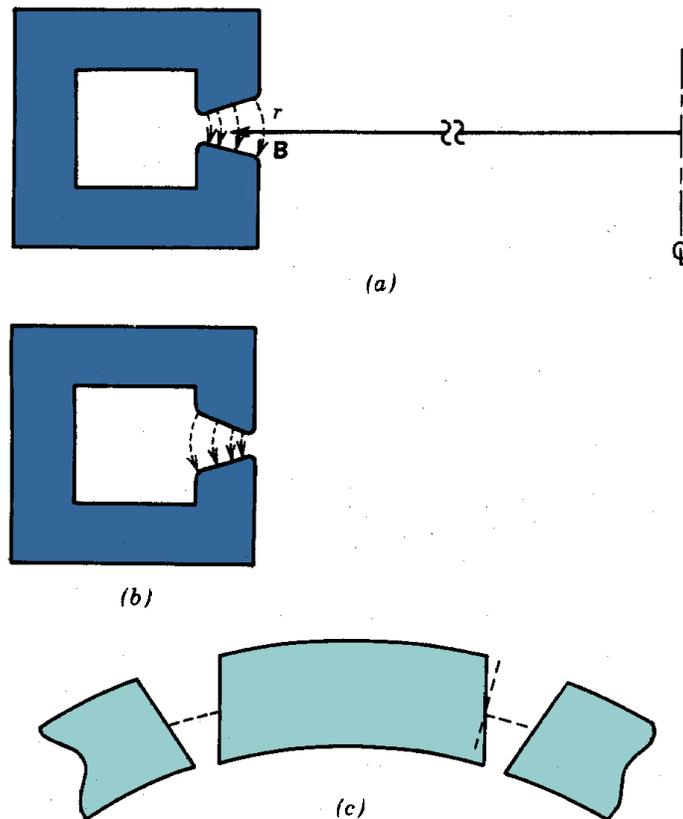
**Figure 15.16** Synchrotron Magnets. (a) Magnet in alternating-gradient synchrotron with strong radial focusing and vertical defocusing. (b) AGS magnet with strong vertical focusing and radial defocusing. (c) Overhead view of uniform-field sector magnet boundaries in zero-gradient synchrotron.
