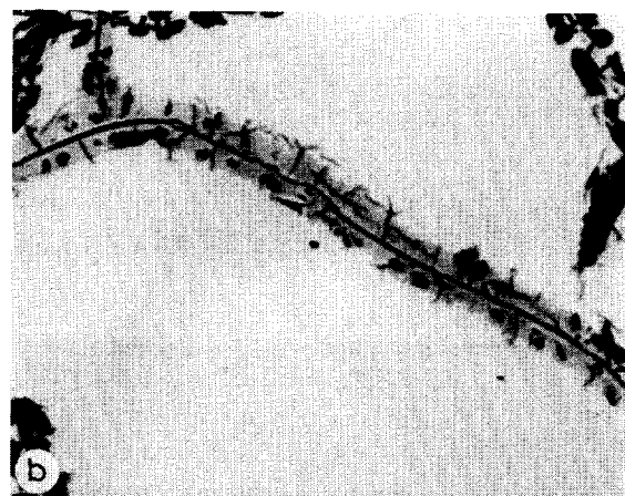
Fig. 4. (a) BEI photograph of a part of partially oxidized grain in sample A. Fine cracks seem to be developing from the rim to the \beta - \gamma_1 boundary. The directions of crack development are almost perpendicular to the phase boundary and the crack edges at the boundary tend to branch along the boundary. At these branching area, \gamma_2 phases develop and make the seed-leaf-shaped structure. The bar is 10 \mu\text{m} long. (b) BEI photograph of a central part of the oxidized grain in sample A. The \gamma_1 phase develops along pre-existing cracks. Fine cracks develop perpendicular to the pre-existing cracks. The bar is 10 \mu\text{m} long.
