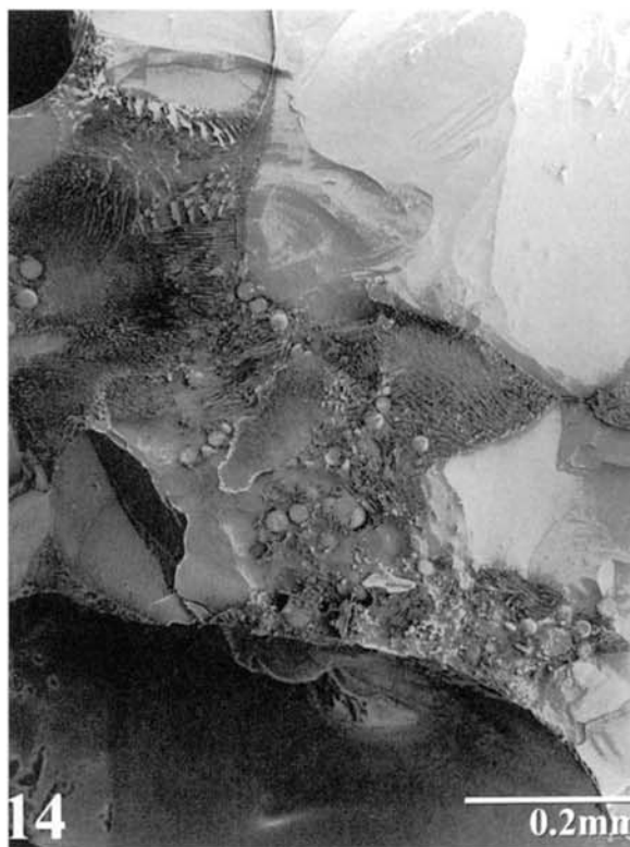
Figure 14. Fractured surface of melting snow. Sample was also etched to sublime the surface water-ice. This procedure reveals the presence of small spherical bodies believed to be a green alga, possibly Chlamydomonas nivalis .
