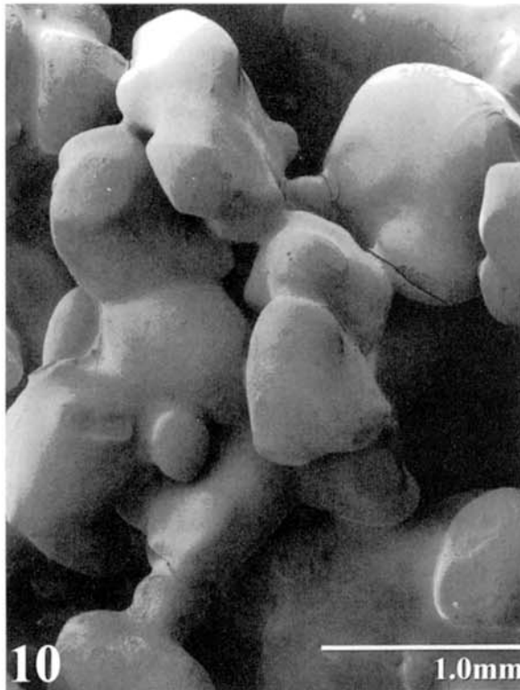
Figure 10. Rounded and well-bonded snow crystals that result from long exposures to low temperature gradients. Sample was collected from a snowpit 19 cm below the surface near Loveland Pass, Colorado, elevation 3600 m ASL.
