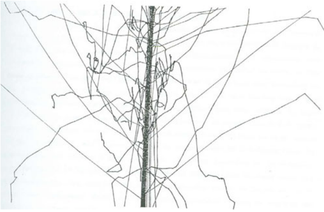
Figure 17. Primary and FSE trajectories simulated by Gauvin (1990) in graphite at 100 keV for a thin foil of 30 nm.
