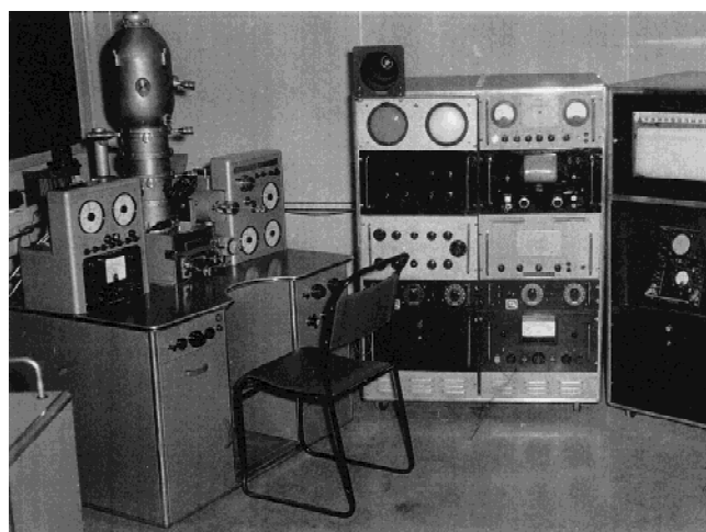
Figure 5. Scanning electron probe microanalyzer for metallurgical use, built at Tube Investments Research Laboratories (TI) in 1959, showing the column (left) and scanning displays (center).
