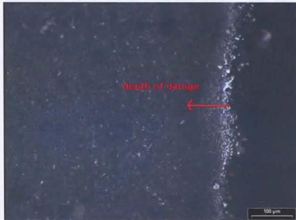
**Figure 5.** Laser-induced heat damage zone.
