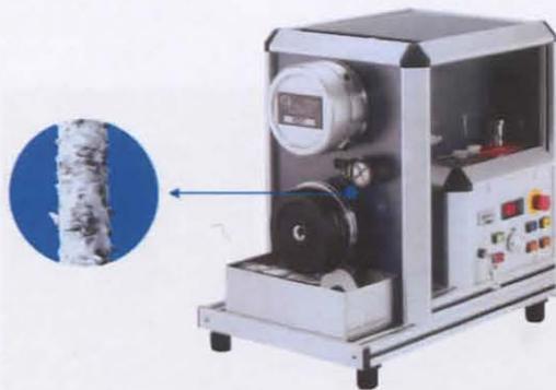
**Figure 3.** Wire-saw.
