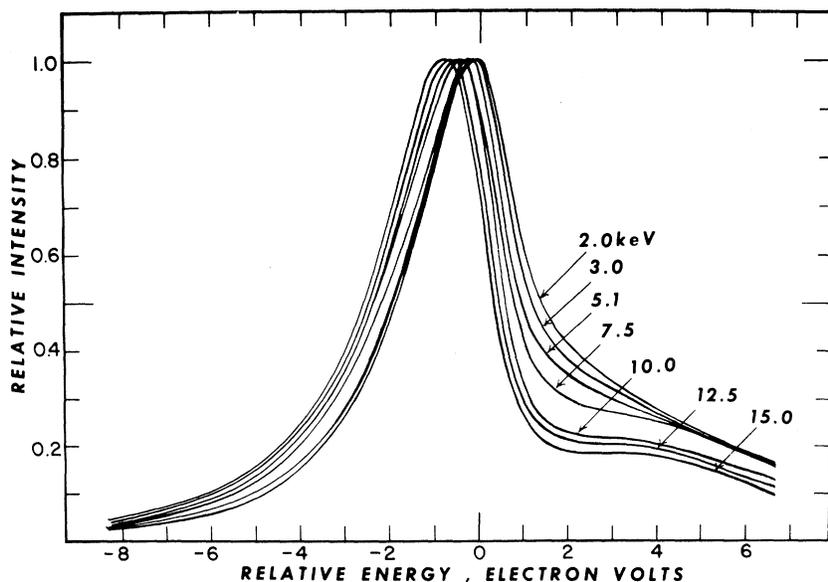
FIG. 1. Ni  $L\alpha$  line profiles for several bombarding electron energies.
