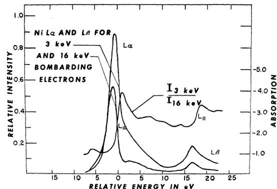
FIG. 3. Ni  $L$  self-absorption spectrum obtained from the ratio of the intensities of the emission spectra in the Ni  $L\alpha$ - $L\beta$  region for 3- and 16-keV bombarding electrons.
