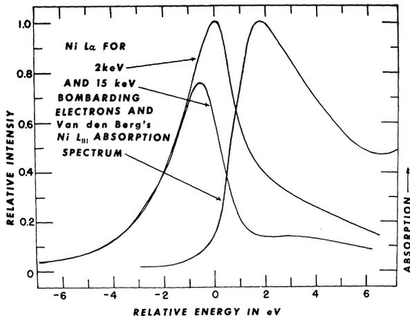
FIG. 2. Apparent coincidence of the observed minimum on the high-energy side of Ni  $L\alpha$  line recorded for 15-keV bombarding electrons with the maximum of  $L_{III}$  absorption spectrum of Ni.
