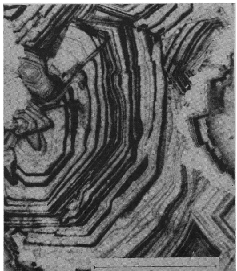
Fig. 1 (above left). Calcite infilling in dolomite. The top photograph was taken by luminescence from the specimen only. The bottom photograph is of the same region of the same specimen, taken with crossed Nicols. All the luminescence photographs are negatives. The dark areas correspond to bright luminescence and the light areas to dim luminescence. Fig. 2 (above right). Calcite infilling in dolomite. A region as photographed by luminescence (top) and with crossed Nicols (bottom). Fig. 3 (below left). Calcite infilling in dolomite. A region as photographed by luminescence (top) and with crossed Nicols (bottom). Fig. 4 (below right). Calcite infilling in dolomite. This photograph was taken by luminescent light, using higher magnification. Under the microscope this single grain revealed 50 distinguishable growth bands.
