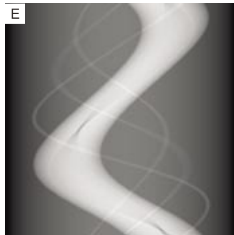
FIGURE 2. This figure shows how computed tomography works. A virtual phantom is shown in A, representing a slice through a core of matrix material (dark gray), with a garnet porphyroblast (mid-gray) and several Fe oxide grains. The garnet has inclusions of matrix material and an Fe oxide. Third-generation scan geometry is shown in B. (C) The raw data profile for the view in B. (D) This shows the data from B after filtering is applied to enhance edges before reconstruction. (E) This is a sinogram of all the data from 512 detectors (columns) and 512 views (rows) for the phantom in A. Zones of higher attenuation (garnet, Fe oxides) are represented by lighter shades of gray. All of these simulations were made using CTSim ( http://www.ctsim.org ).
