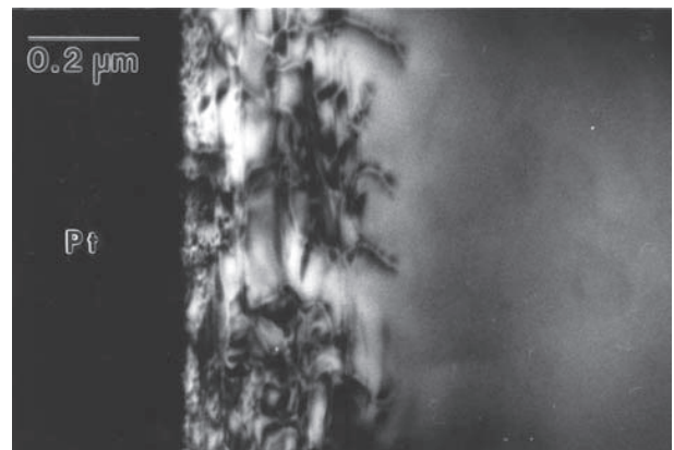
FIGURE 7. A bright-field TEM image of a FIB-milled forsteritic olivine foil showing the defect-rich zone near the surface due to polishing.
