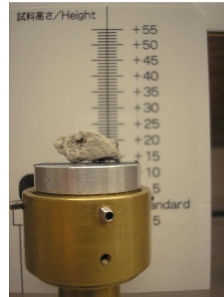
Here is an example of the SAME sample, but on top of DIFFERENT SAMPLE HOLDERS. The "height" you enter in the Hitachi software is DIFFERENT for each case.
