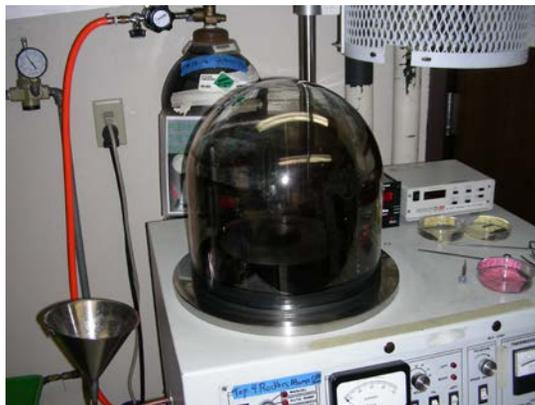
Our lab has the capability to Carbon coat or Iridium coat samples for high vacuum analysis.
