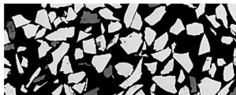
Backscattered electron image of grains of the SMS fayalite reference material. About ten per cent of the grains are a darker gray color. Preliminary data suggest the impurity is an amphibole, possibly grunerite, a mineral found associated with the fayalite from Rockport, Massachusetts chosen to
