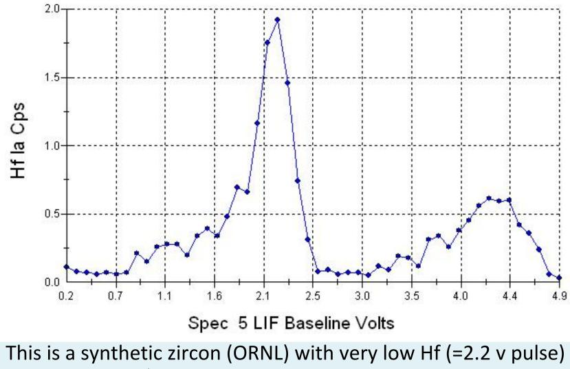
and with the 2<sup>nd</sup> order Zr La pulse having ~30% of its intensity.
