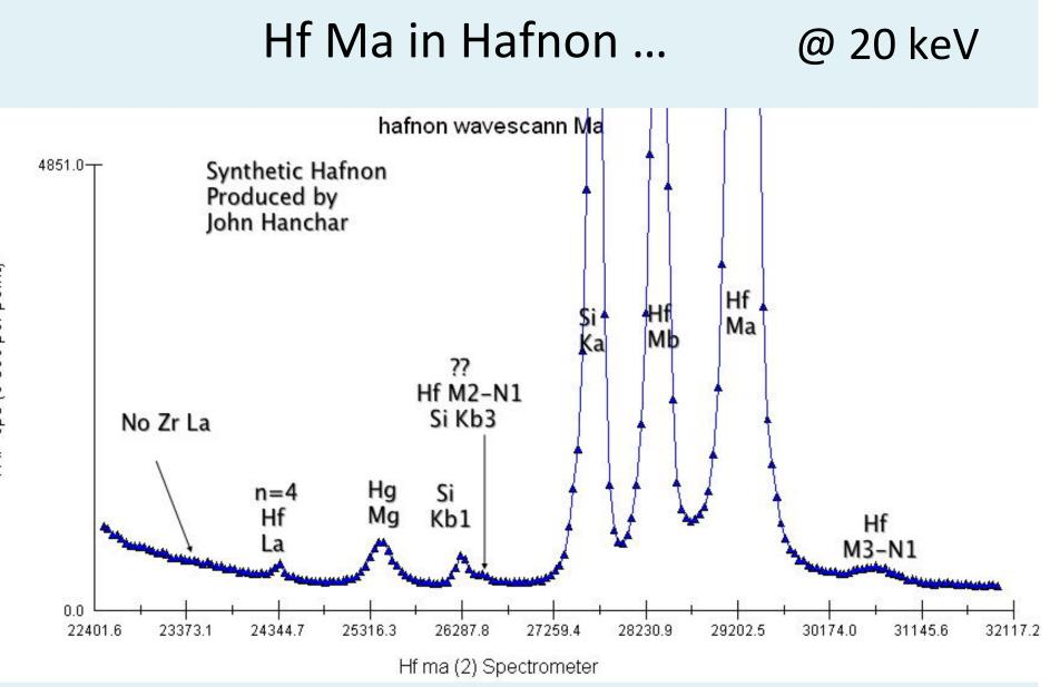
Hf Ma sits at low end of spectrometer where the background is curved....
