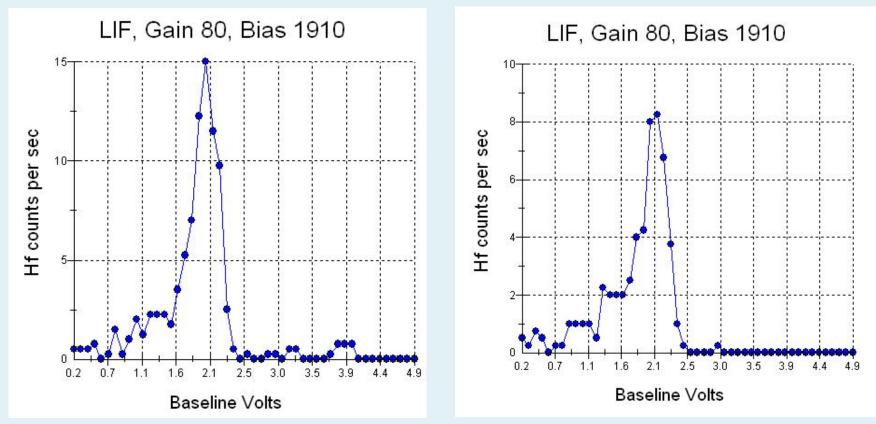
91500 at 20 keV. Note 2<sup>nd</sup> order Zr La pulse at 3.9 volts, relative to 1<sup>st</sup> order Hf Ma pulse at ~1.95 volts 91500 at 17 keV. Note no 2<sup>nd</sup> order Zr La pulse at 3.9 volts
