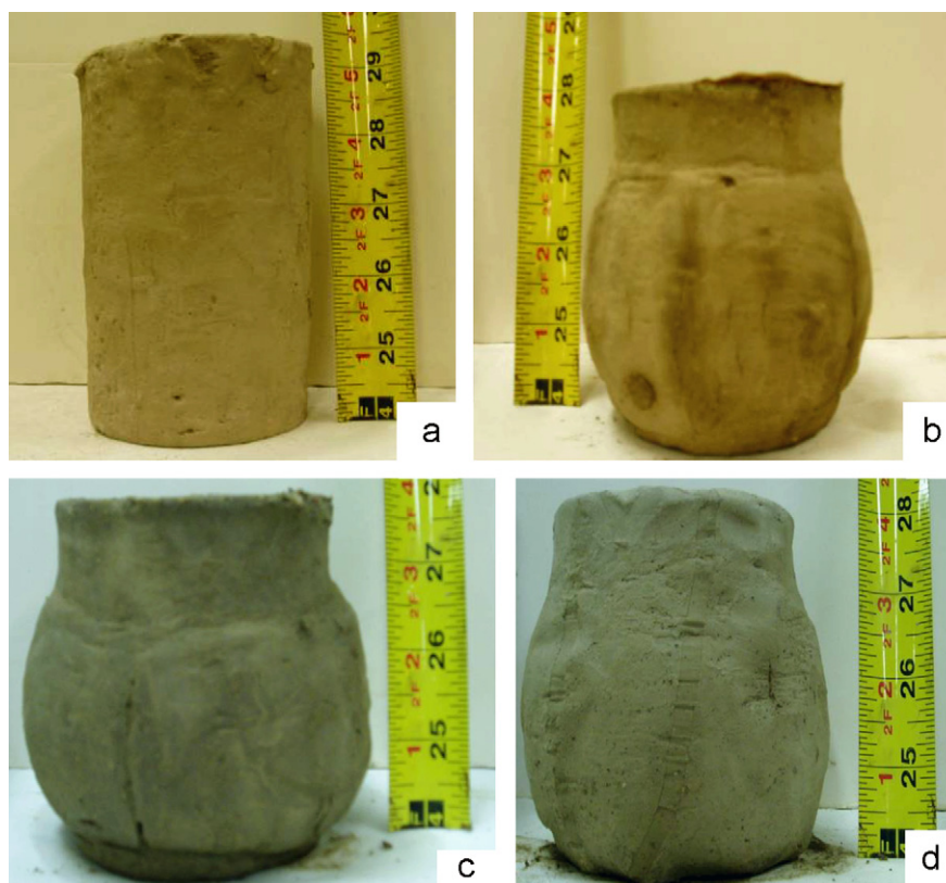
Fig. 7. Photographs of CTC test samples: (a) before the test; and (b), (c), (d) after test; (b) for Sky Pilot; and (c) and (d) for Tiskilwa Till.
