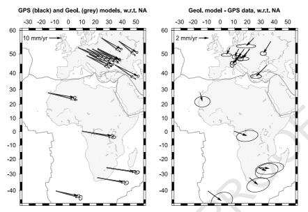
Fig. 4. (Left) Predictions of geologic and geodetic NU–NA and EU–NA angular velocity vectors at GPS sites from the Nubian and Eurasian plates. North American plate is fixed. (Right) Residual velocities of GPS sites on the Nubian and Eurasian plates
