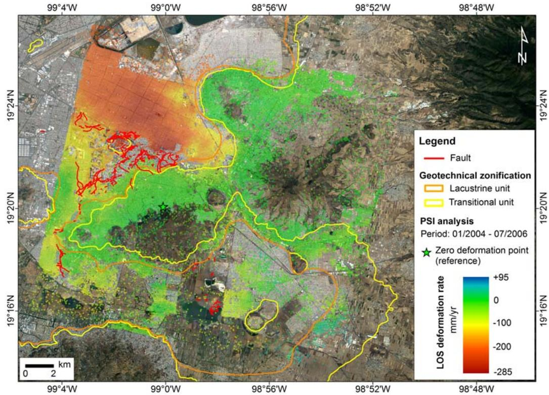
**Fig. 2** Persistent Scatterer InSAR (PSI) displacement map of the southeastern sector of the Mexico City Metropolitan area overlapped onto high-resolution satellite imagery. Faults in the Iztapalapa and Chalco areas are modified from CMFS (2008) and Ortiz-Zamora (2007), respectively. Geotechnical zonification after GDF (2004).
