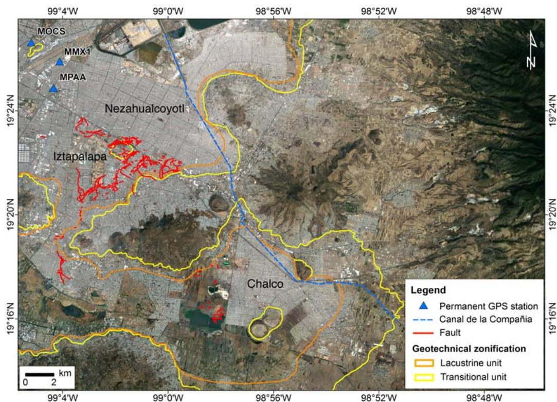
**Fig. 1.** Satellite image showing the location of study area. Faults in the Iztapalapa and Chalco areas are modified from CMFS (2008) and Ortiz-Zamora (2007) respectively. Geotechnical zonification after GDF (2004).
