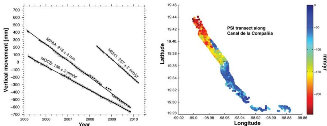
**Fig. 4.** Left: Vertical time series for MMX1, MRRA and MOCS permanent GPS sites; see Fig. 1 for site location. Grey dots are daily solutions and black dots averaged weekly solutions. Right: Retrieval of PSI points (Fig. 2) along a 250-m wide transect centred on the Canal de la Compañía (see Fig. 1 for location).
