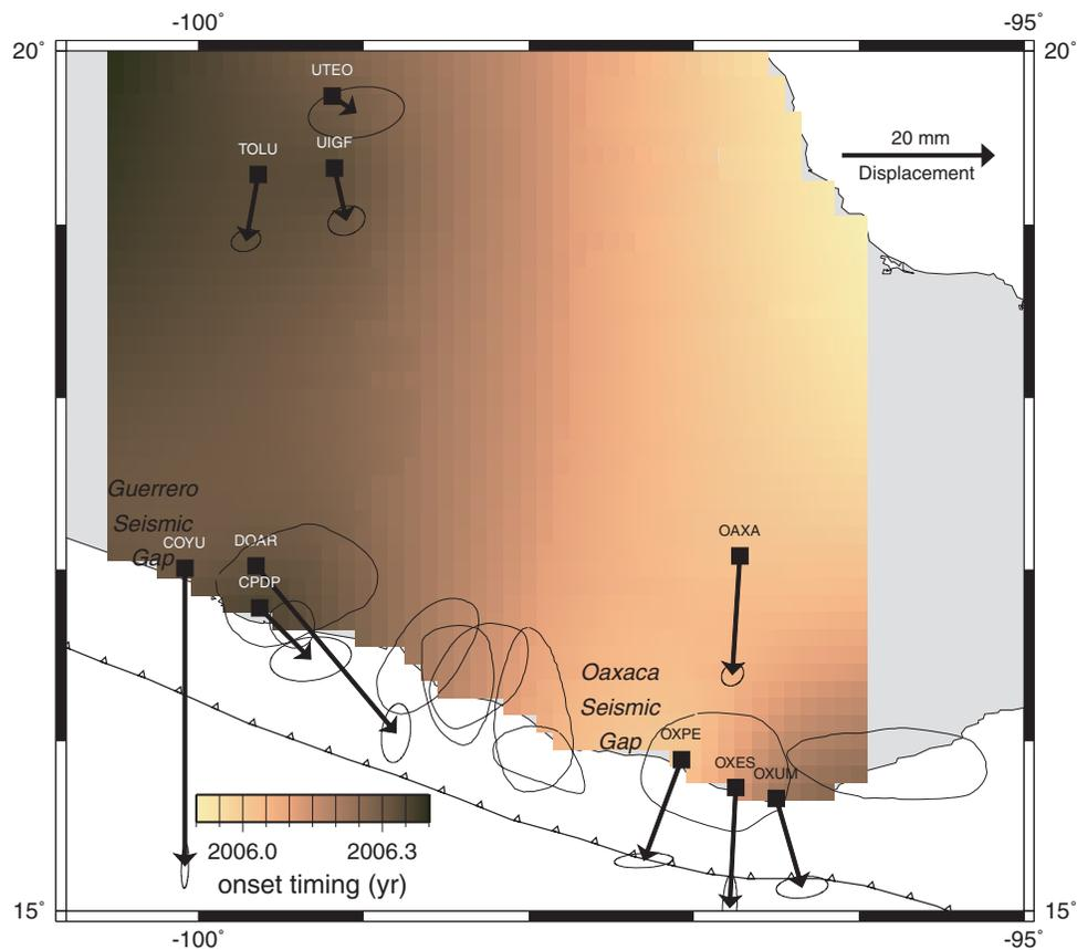
**Figure 10.** Vector displacements and timing of the 2006 transient episode from hyperbolic tangent fits to GPS coordinate time-series shown in Fig. 9. Site motions are specified relative to the North American plate.
