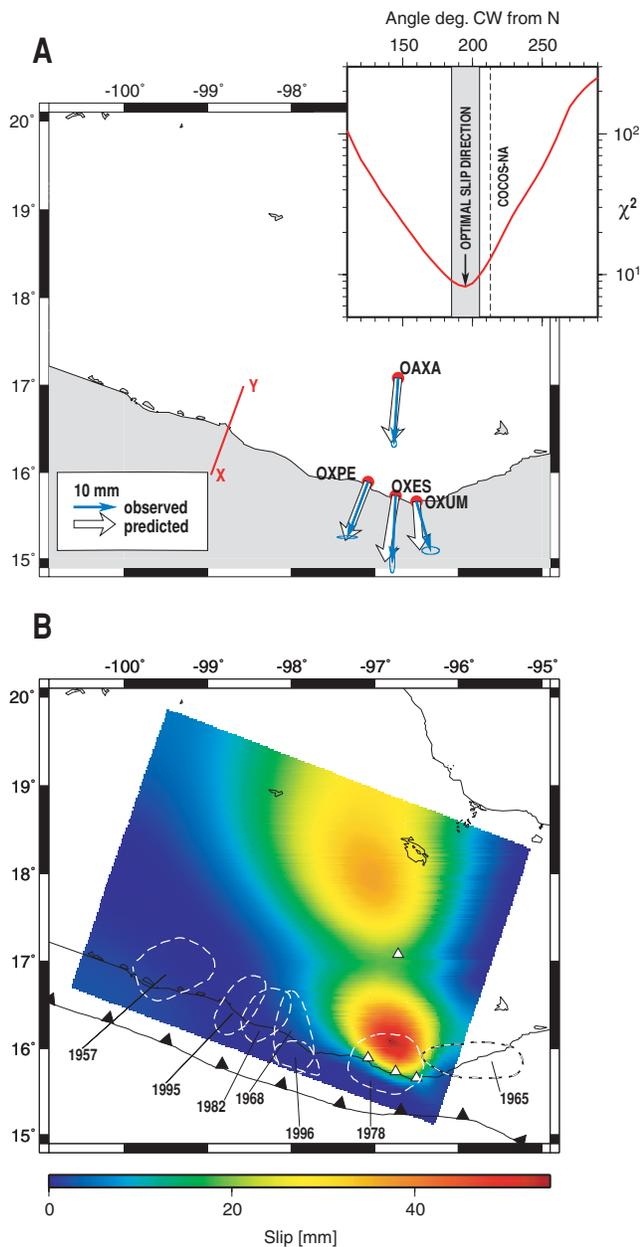
**Figure 11.** Inversion results for the 2006 transient slip event. Layout is as in Fig. 7. (a) Observed and estimated offsets with uncertainties. (b) Location and magnitude of transient slip. Triangles indicate locations of GPS stations in the Oaxaca region that are inverted for the 2006 transient slip event.
