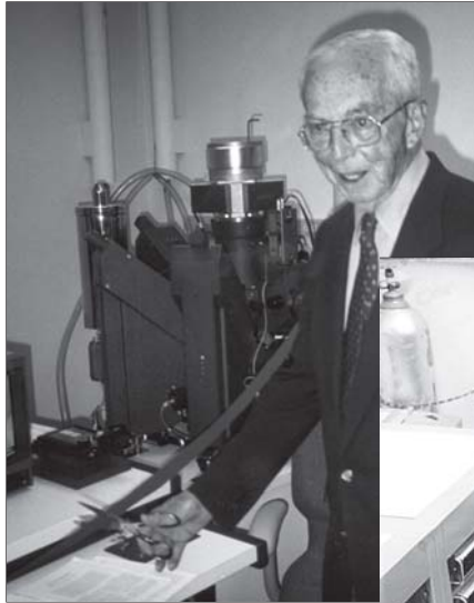
Left, Gene Cameron at the opening of the new probe lab in 1993, and below, Gene operating the UW's first electron microprobe, a hand-operated, three spectrometer ARL-EMX. He purchased the instrument in 1966.
