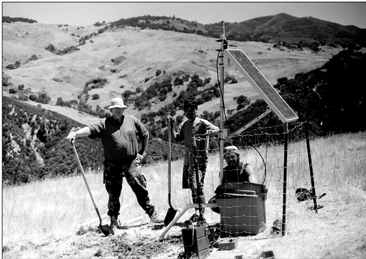
Kyle Roberts, Haijiang Zhang and Karl Rittger installing the last real-time telemetered seismic station for Cliff Thurber's seismic field project near Parkfield, CA. Photo by Neal Lord.
