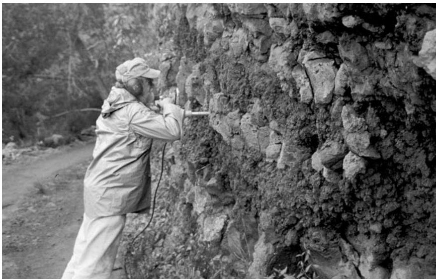
Figure 1. Ken Hoffman drilling to collect oriented core samples from a lava flow sequence on La Palma, Canary Islands, in January 2000. These particular lava flows have been ^{40}\text{Ar}/^{39}\text{Ar} -dated at 579,000 years before the present and were found to record the Big Lost excursion shown Figure 2. (Brad Singer)
