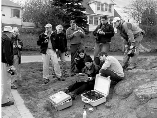
Hill Street, Thunder Bay, Ontario, tsunami deposit. The field XRD suitcase was a big hit wherever we went. Here we analyze clay minerals from devitrified volcanic glass.
