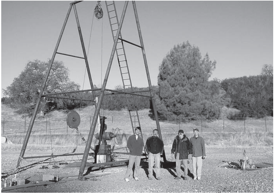
The main phase of deep drilling at SAFOD ended in the summer of 2006. What remains is a frame and winch system used to install and retrieve borehole logging tools and seismic instruments that are periodically placed in the SAFOD borehole. Standing in front of the A-frame are (left to right) grad student Riley Gannon and co-PI Steve Roecker of RPI, Lee Powell, and Yunfeng Liu. (Cliff Thurber)
