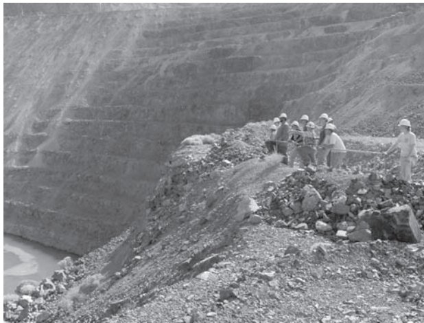
Left, Day 3: A geologist at Newmont's Phoenix mine describes the local geology at an overlook of a mined out pit and its associated pit lake, visible in the lower left corner of the picture. Each step in the wall in the background is approximately 20 feet.
