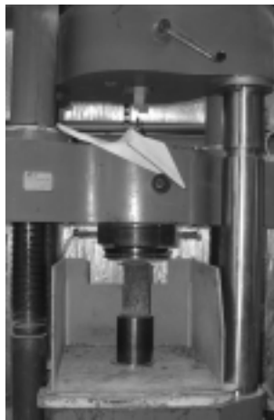
Figs. 7a, 7b. As floors were poured concrete samples were tested in an independent lab.
