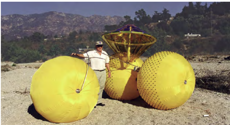
Fig. 14.1 Original 3-wheeled inflatable rover shown with inventor, Jack Jones, NASA Jet Propulsion Laboratory (Jones et al., 1999).
