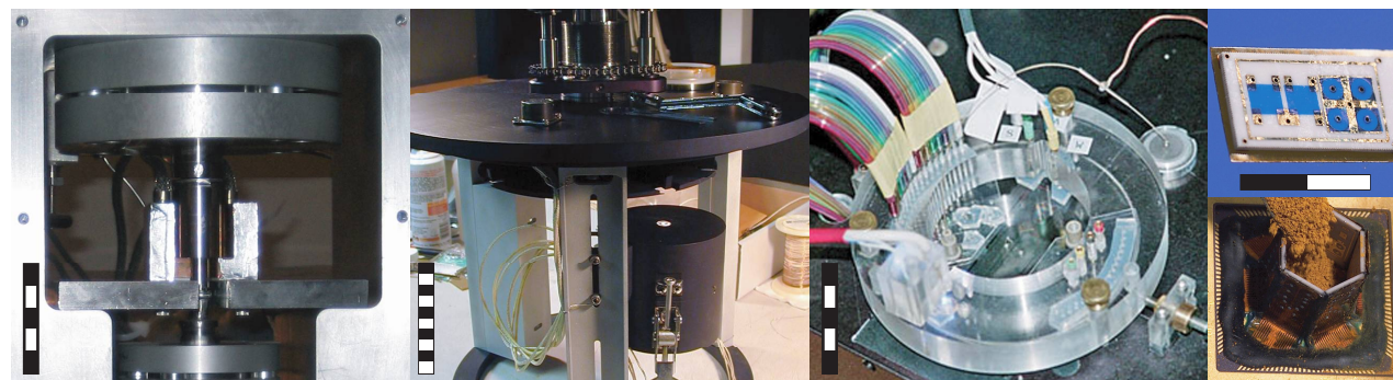
FIG. 4. Concept illustration of Urey —Mars organic and oxidant detector (images courtesy NASA-JPL) and photographs of field subsystem prototypes (scale bar graduations ~1 cm): (A) Sub-Critical Water Extractor, (B) Mars Organic Detector, (C) \mu -Capillary Electrophoresis instrument, and (D) Mars Oxidation Investigation deck unit (top) and internal unit (bottom).
