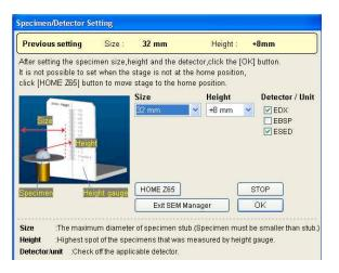
Note 2: Hitachi's graphic (left) is confusing. It incorrectly suggests you are measuring the (vertical red line) height of the specimen, when you are not! You are measuring the TOTAL height of the holder+sample.... otherwise, how could you have a negative sample height! Note 3: DO NOT touch the green check boxes for "detector/unit". Leave them alone as they are. We have to "trick" the software as it is not totally correct for our detector setup.
