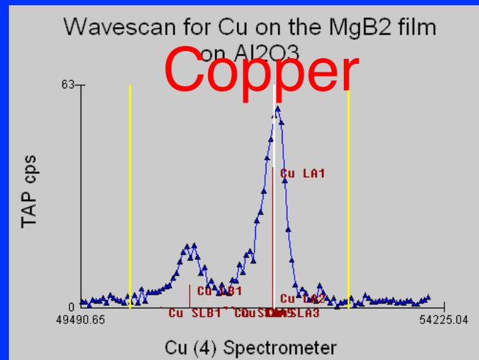
Over months of study, many unexpected elements turned up, generally from the sputtering process: the Ar atmosphere, Cu from sputtering holder, C from “pure B sputtering target” (B<sub>4</sub>C, manufacturer didn’t think C counted as an element!).
