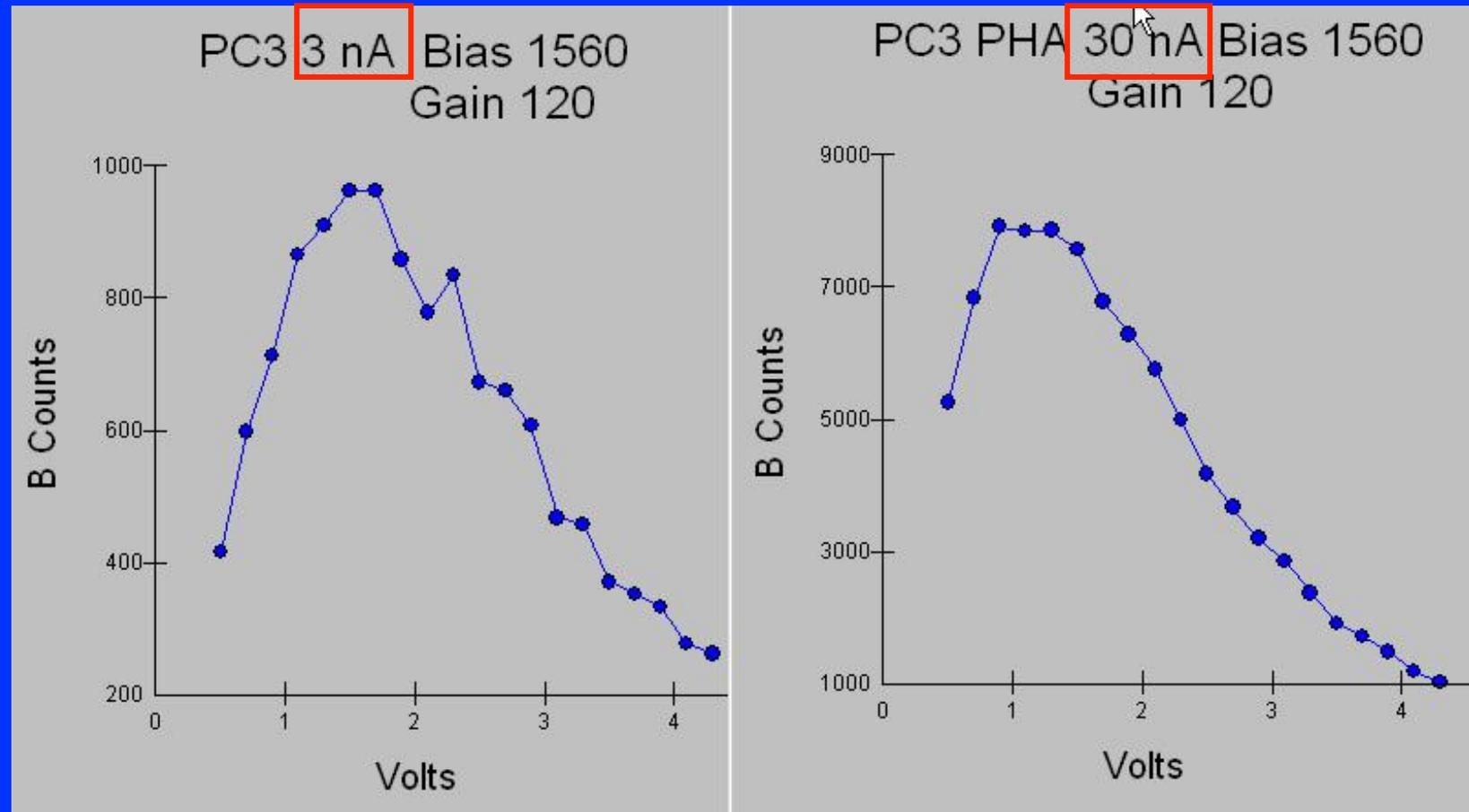
– Calibrate on B with low current (1-3 nA), then do acquisition at 30 nA)
